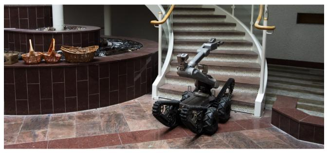
Figure 5: A bomb disposal robot facing a staircase. Photo courtesy of the Swedish Police Authority.
